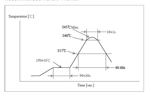
Pre heating temperature:  $150\pm10[^{\circ}\mathbb{C}]$  Pre heating time:  $90\pm30[\sec.]$  Heating temperature:  $240\pm5[^{\circ}\mathbb{C}]$  Heating time:  $10\pm1[\sec.]$
